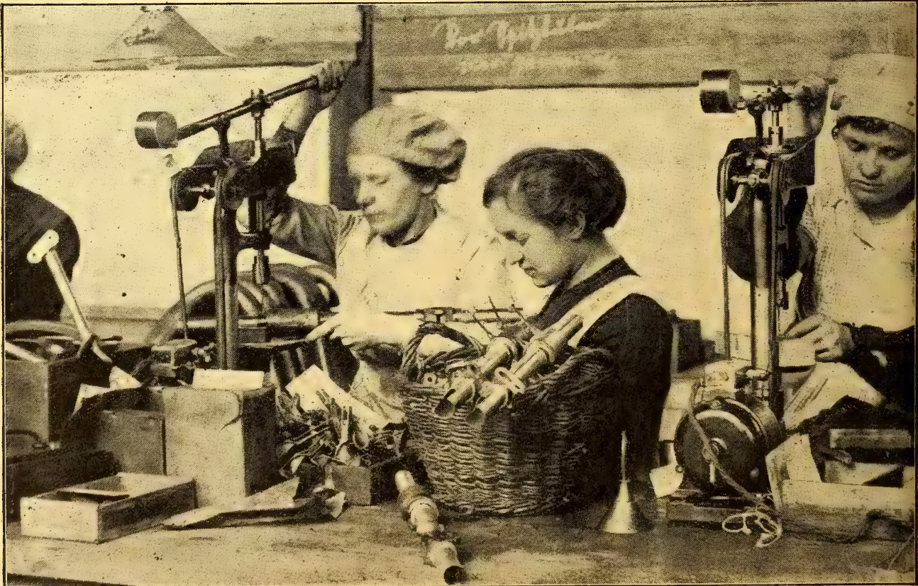
GERMAN AIRCRAFT PRODUCTION.—Drilling small parts with a very neat form of electric sensitive drill. One does not notice any evidence of acute starvation. The chalked notice at the back means "Beware of Pick-pockets," which may imply inherent moral obliquity among the working classes, or may be only a joke, or may be an evidence of acute starvation.
